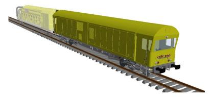
A sketch of the battery wagon that complements the traditionally diesel-powered versions of the railway specialist Railcare's machines. Emission-free battery-powered vehicles improve the working environment and increase the potential for use in underground projects, for example in subways and mines. © 2019 Railcare Group AB
