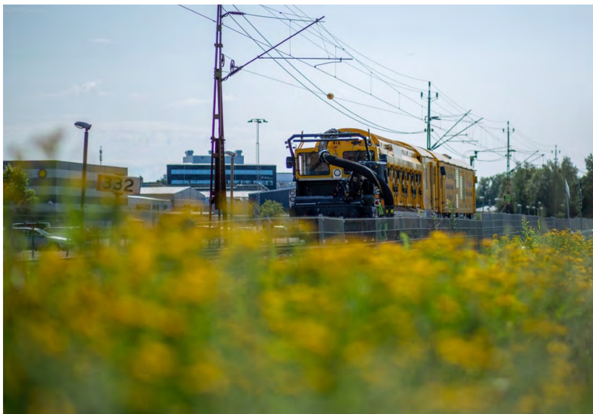
Multi Purpose Vehicle. The world's first and largest battery-powered maintenance machine for railways.
